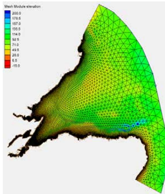
**Figure 5.11.** Example of a wave transformation model grid such as might be used to look at the effect of wave dissipation measures.
