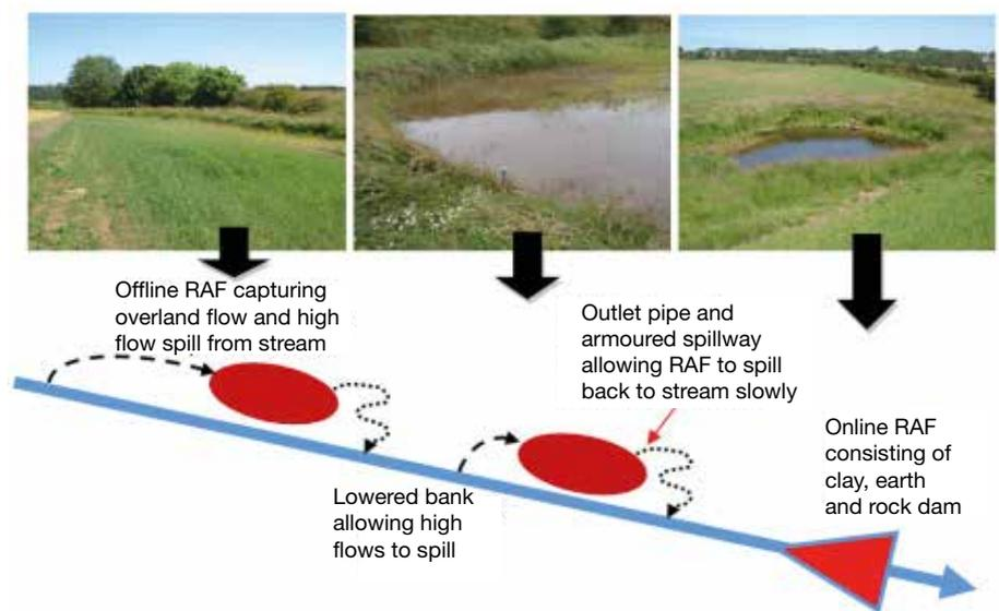
Figure 2.32. Offline storage areas and other attenuation features (Runoff Attenuation Features) constructed in the Belford Burn catchment, Northumberland (from Wilkinson et al.<sup>61</sup>).
