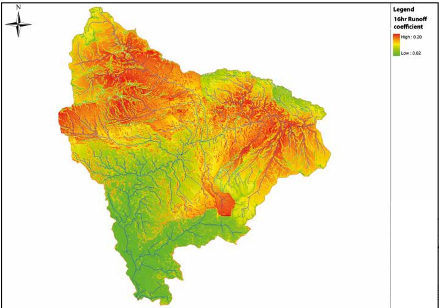
Figure 5.7. Generation of runoff that contributes to the flood peak in the Allan Water catchment, Stirlingshire: This figure shows that the majority of runoff contributing to downstream flooding is generated in the north-west of the catchment and hence where runoff reduction measures would have most effect (from CRESS and Halcrow<sup>122</sup>).
