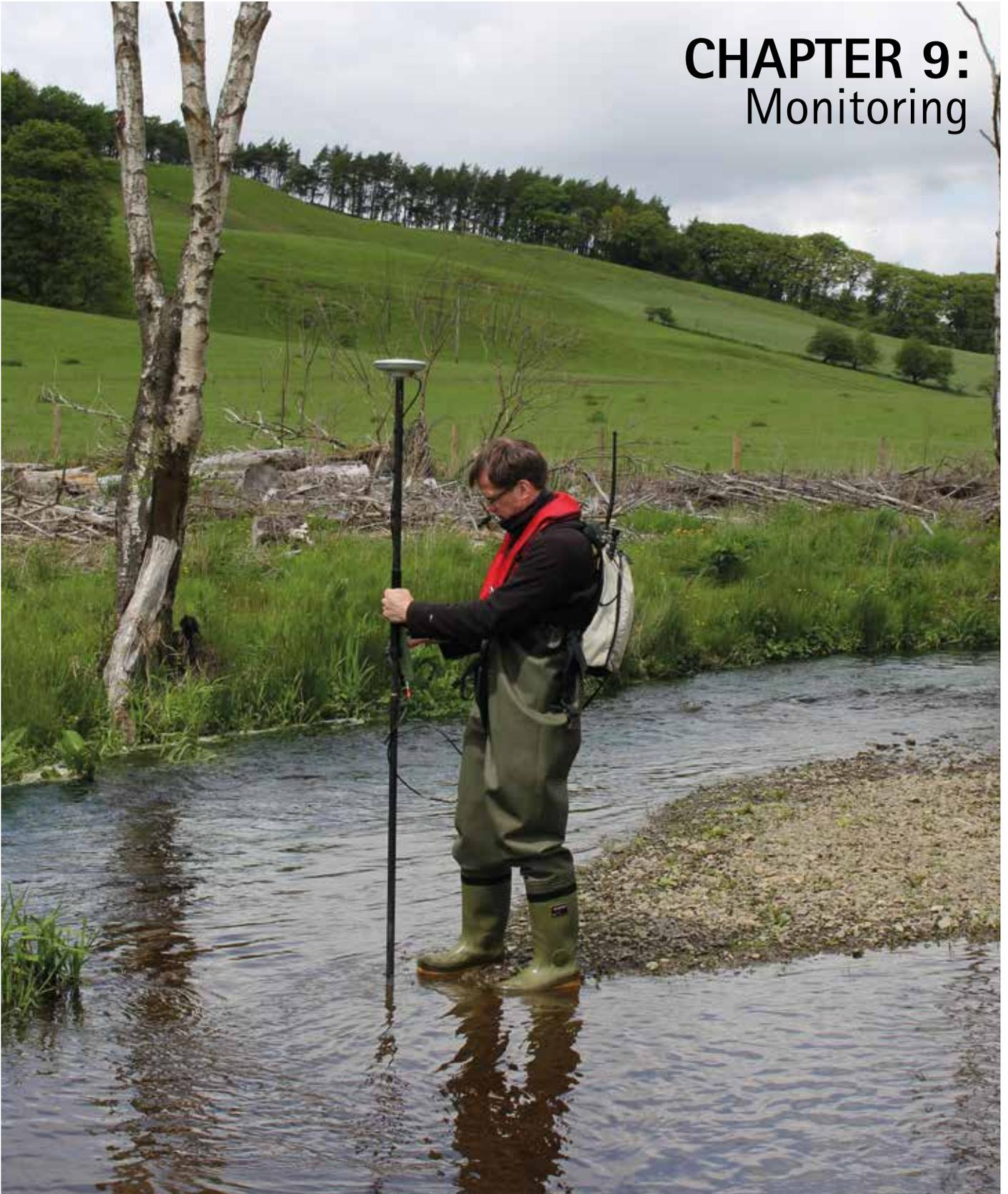
Figure 9.1. Cross section surveying on the Eddleston Water, Scottish Borders (© C. Spray).
