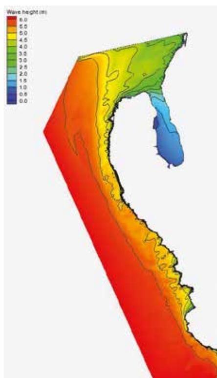
Figure 5.2. Example of wave transformation model output for the Rhins of Galloway showing how wave heights change as they move inshore from a south-westerly direction (from the Solway Firth Flood Forecasting System Report, JBA Consulting, 2015).
