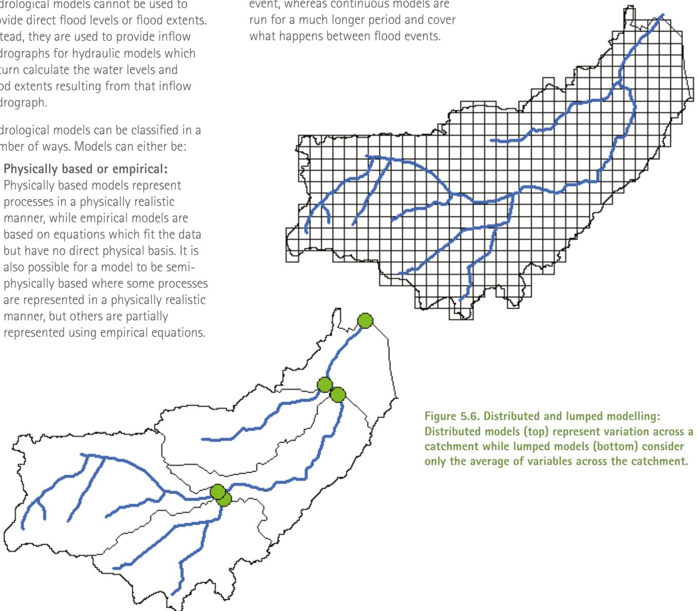
Figure 5.6. Distributed and lumped modelling: Distributed models (top) represent variation across a catchment while lumped models (bottom) consider only the average of variables across the catchment.
