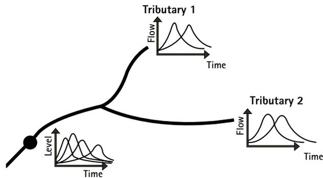
**Figure 5.10. Scenario testing using a hydraulic model which has inflows at tributaries 1 and 2: In this example a series of model runs are carried out shifting design hydrographs for tributary hydrographs earlier and later in time and the impact on peak stage at a receptor further downstream is investigated. Other scenarios could involve changing the relative magnitude of the tributary hydrographs or changing the hydrograph shape.**
